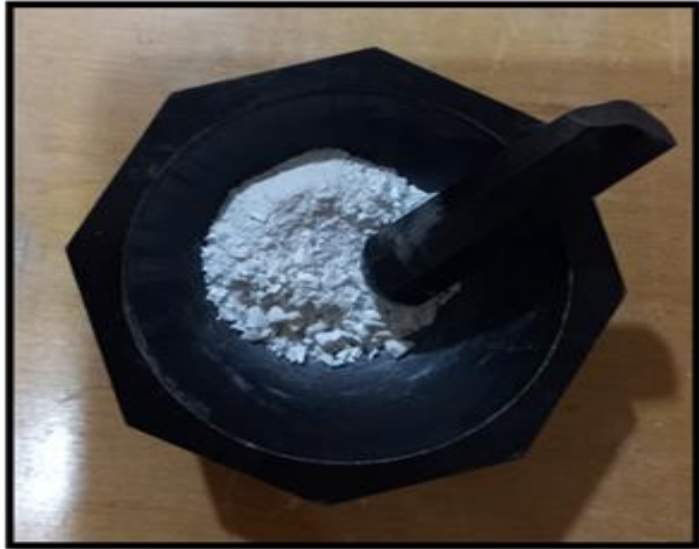
Fig 4.2: Calcinated bone into powder form by mortar pestle
