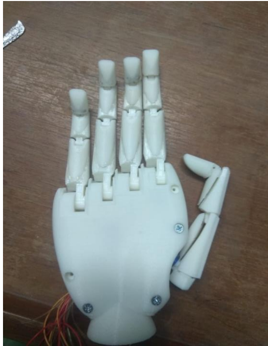
The above image shows the prosthetic arm in the extension position
