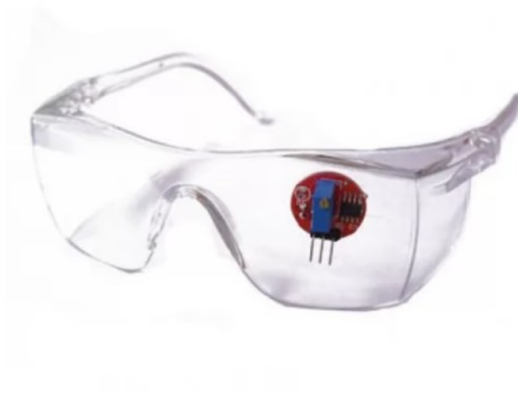
Fig 4.1 Eye blink sensor attached to test goggles
