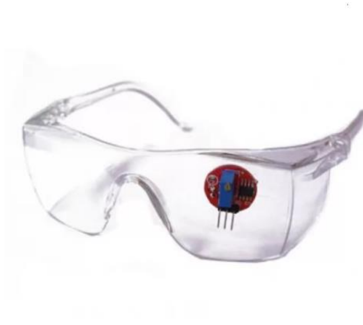
Fig 4.1 Eye blink sensor attached to test goggles
