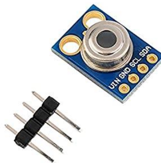
Fig 4.3.MLX90614 Non contact IR temperature sensor
