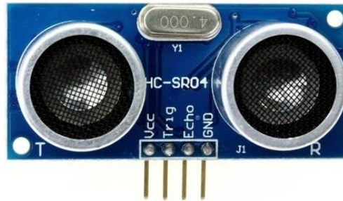
Fig 4.5.HC SR04 ultrasonic sensor
