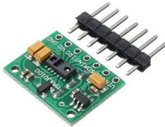
Fig 4.4. MAX30100 pulse oximeter and heart rate sensor module
