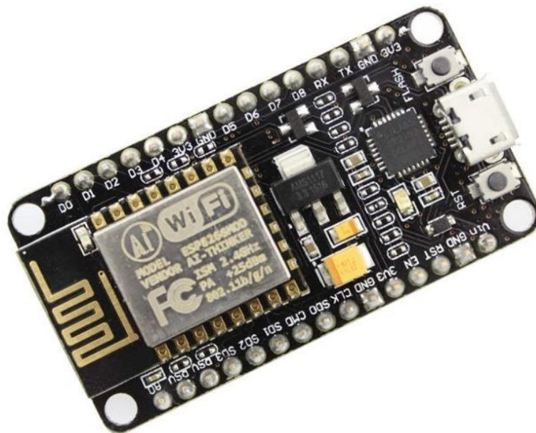
Fig: 2.15 NodeMCU Development Board/kit v1.0 (Version2)
