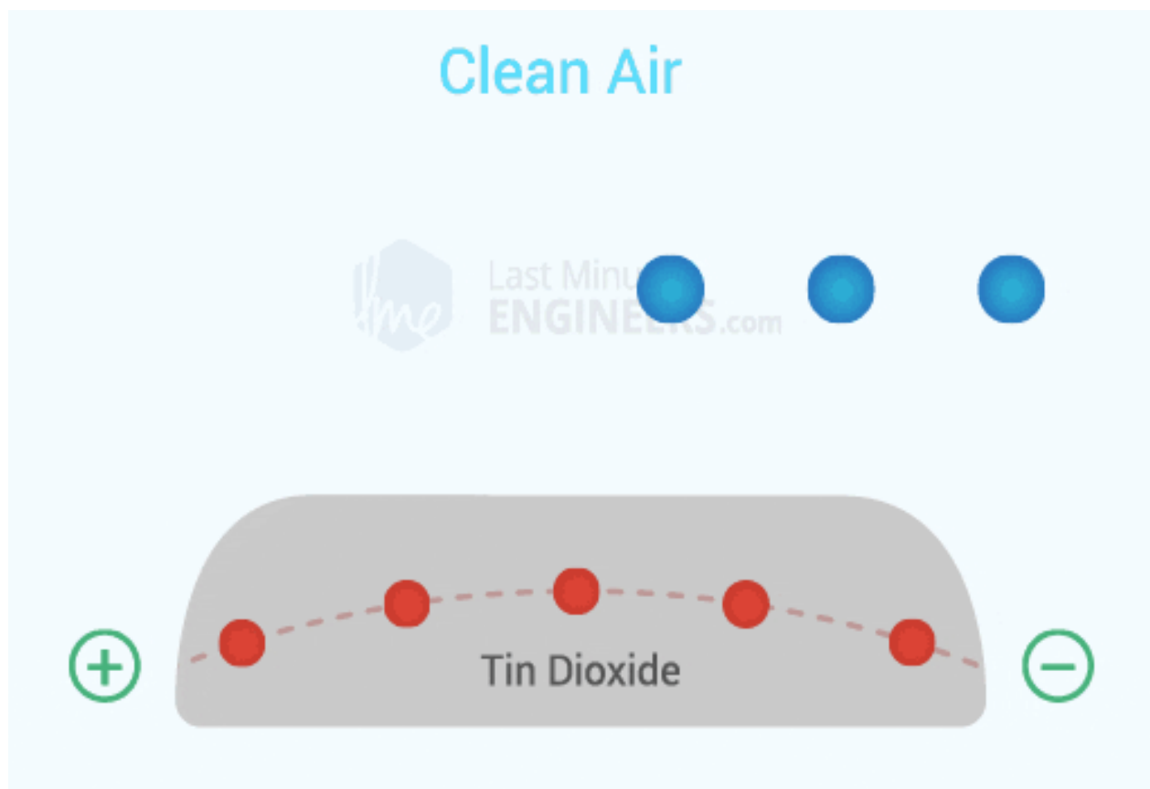
Fig 3.5: Working of Gas sensor
