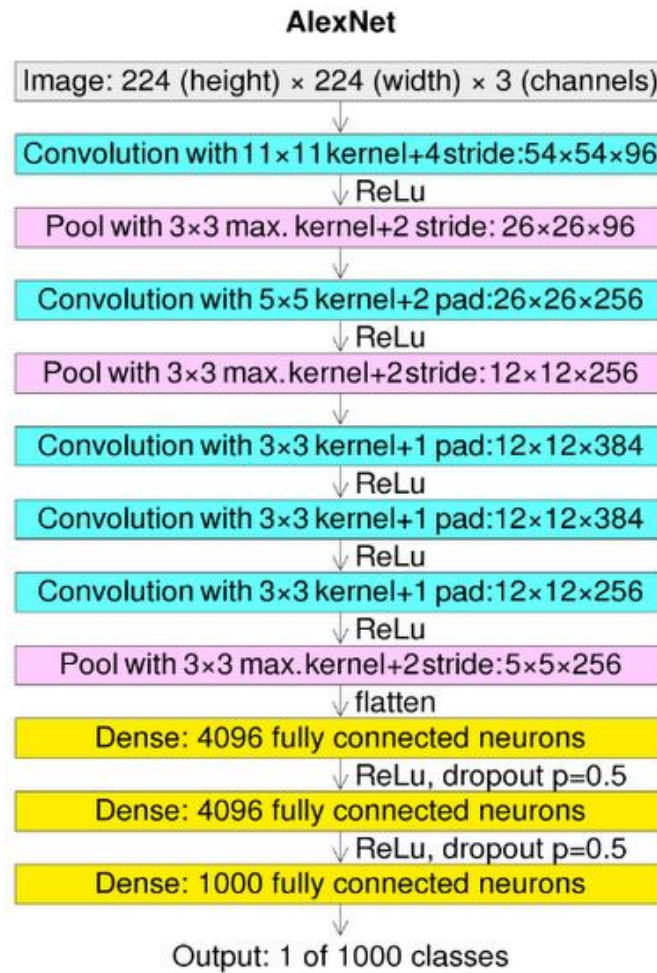
Fig: Architecture of AlexNet
