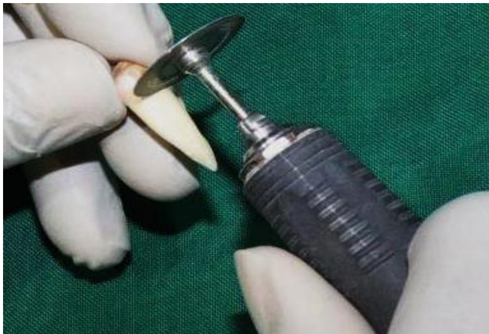
Fig.13 Sectioning tooth samples 15 mm from apex using slow speed handpiece
