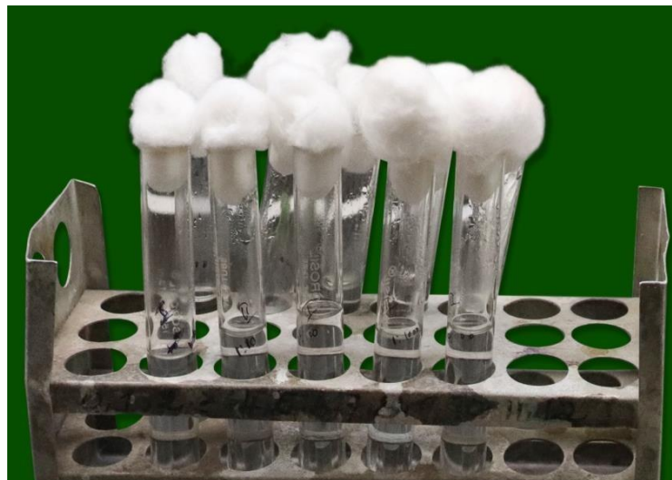
Fig.21 Ten fold serial dilution of samples, inoculated into Mueller-Hinton culture
