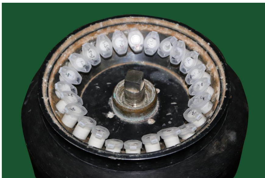
Fig.4 Centrifugation of 3Mix antibiotic paste with barium sulfate
