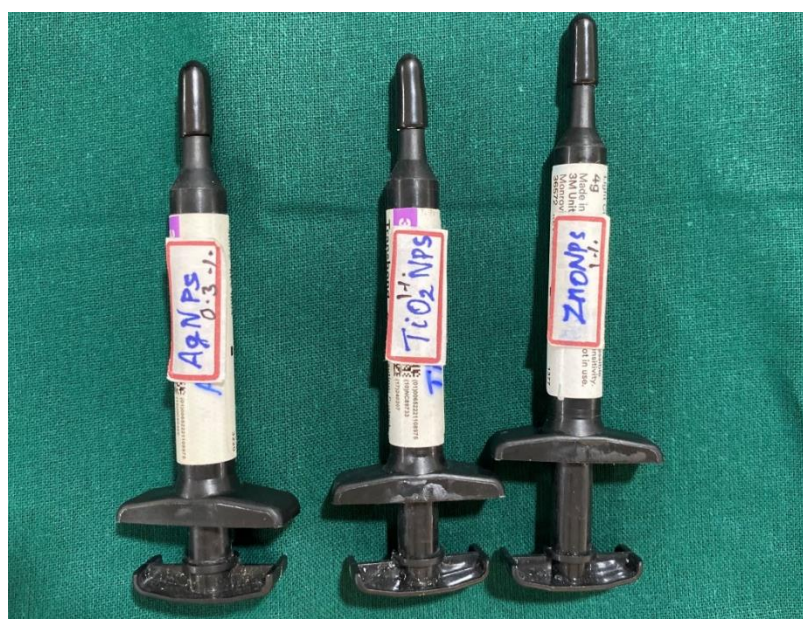
Figure 8: Prepared Nano Adhesives
