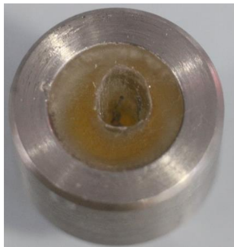
Figure 20b: Cylindrical moulds with acrylic resin – after removal of aluminium foil
