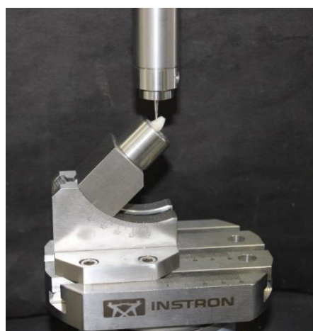
Figure 23: 130° angle to the long axis of tooth
