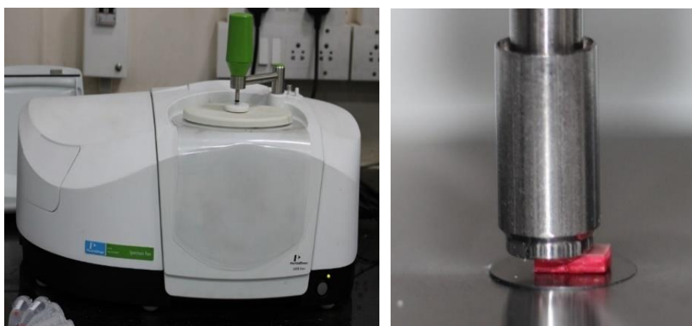
FIGURE 20: a) Spectrum 2 spectrometer b) Sample scanned in ATR mode
