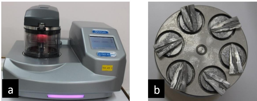
FIGURE 22 a) Sputter coater (QUORUM 150 ET PLUS) b) Sputter coated samples
