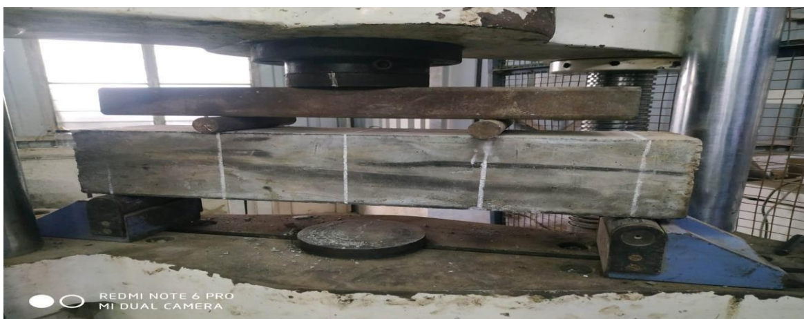
Fig4.7: Testingofflexural beams overtheGFRPwrappingprocess
