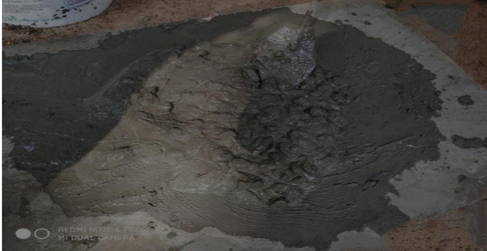
Fig:3.12 M30 Grade concrete mixing in partial replacement of GGBS by cement in 20%, 30%, 40% & 50%.
