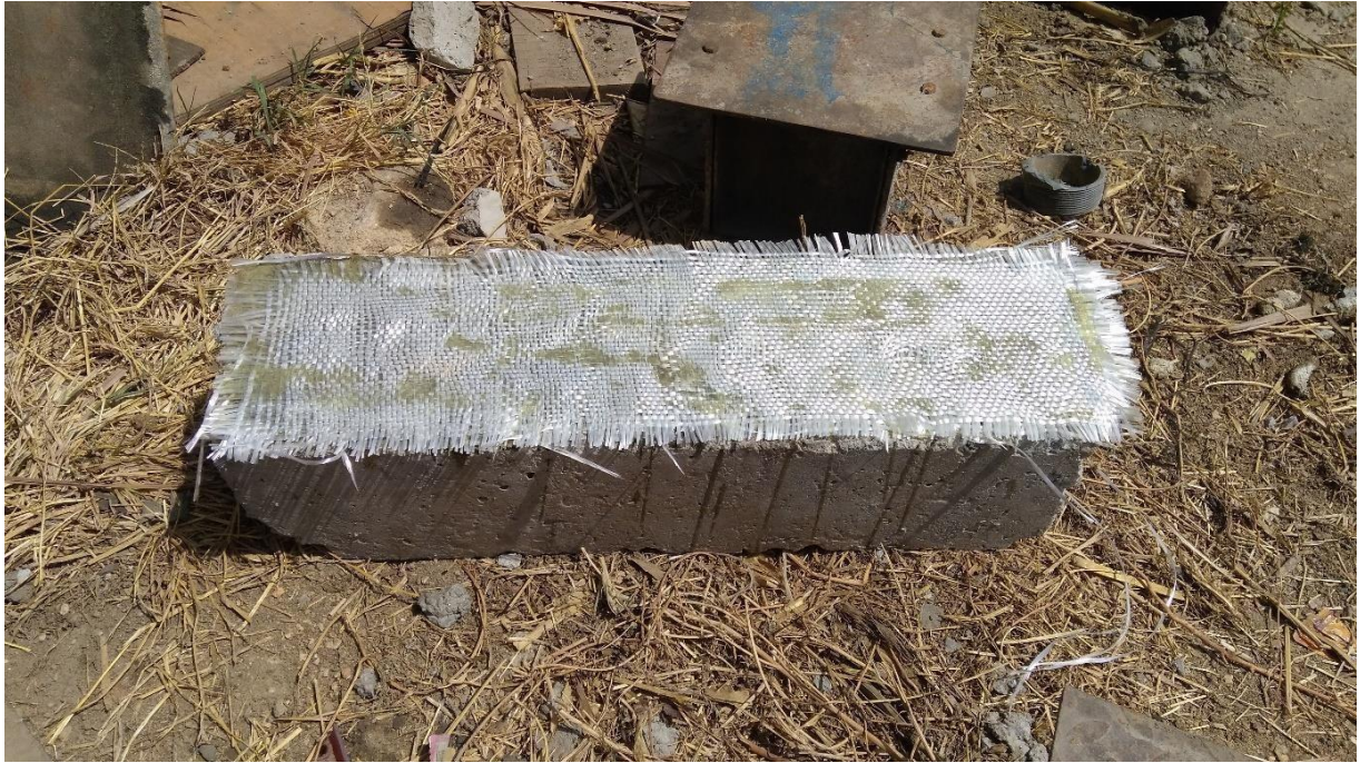
Fig :3.23 After 24 hours the GFRP was fixed in the RC beam
