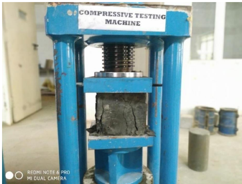
Fig.4.3: Preparation of testing of compression cubes
