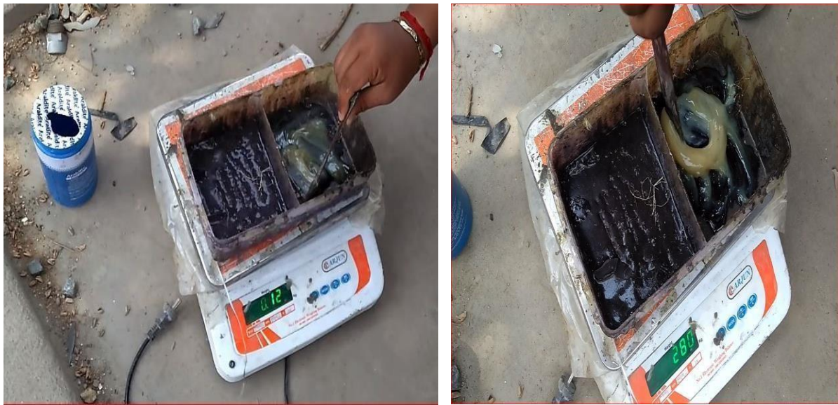
Fig :3.20 Mixing of resin & hardener in 2:1 ratio
