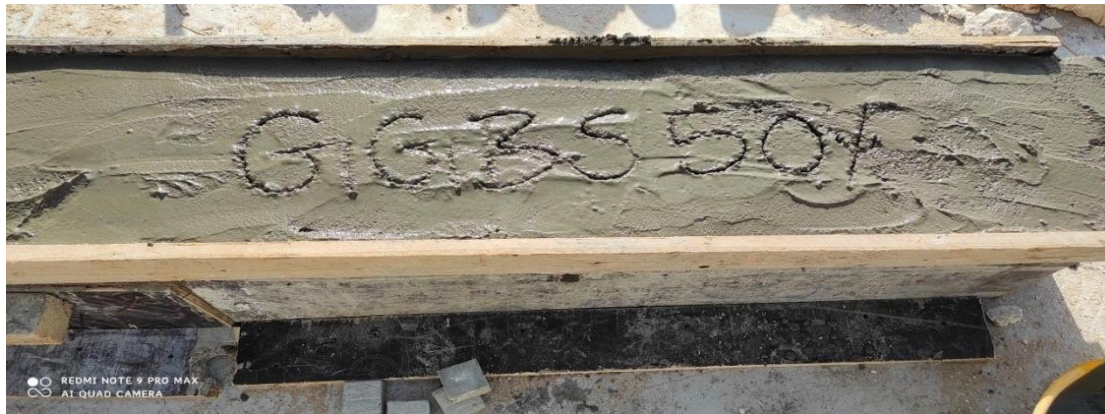
Fig:3.18 Before curing the flexural beams
