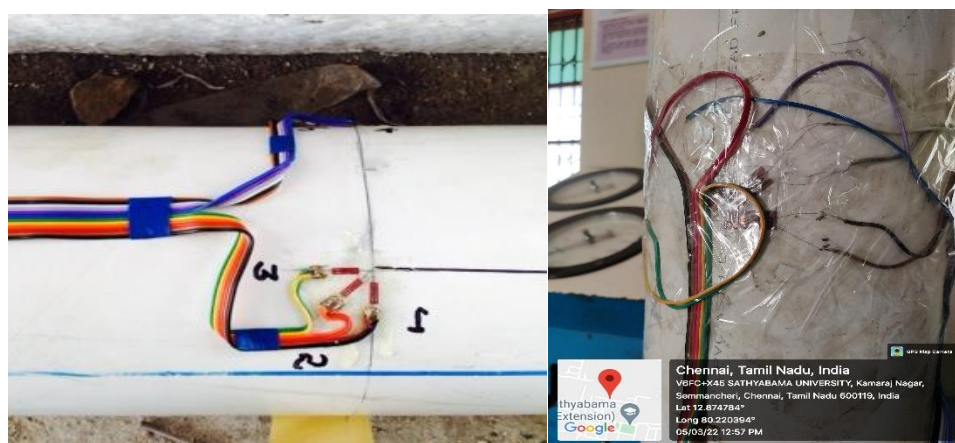
Fig: 4.5: Strain gauge embedded in pipe
