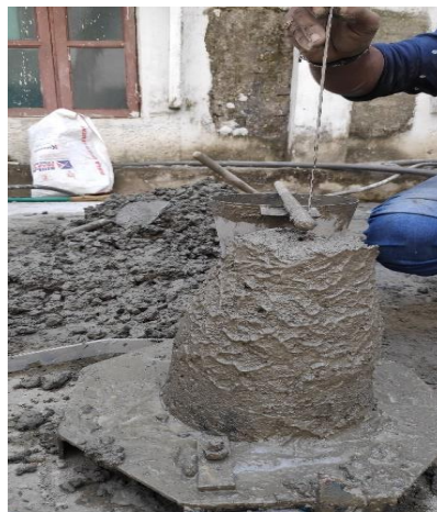
Fig.4.4 Slump cone test
