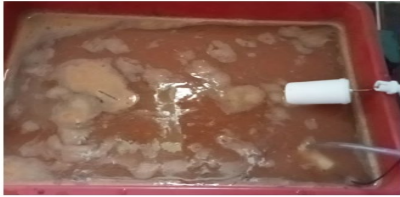
Fig: 4.9 : Water level sensor connected at the field
