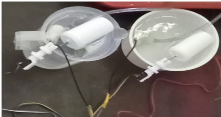
Fig: 4.8 : Water level sensors connected at the water sources (borewell and water tank)
