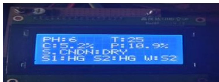
Fig: 5.2 : LCD displaying pH value, nutrient values in the soil, soil moisture condition, level in the water sources, and displaying water taken from the source.
