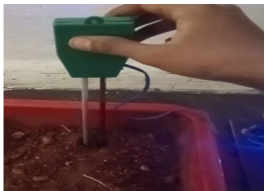
Fig: 4.5 : pH sensor dipped in the soil
