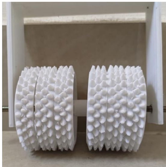
Fig:4.5 : Spiked wheels of Weeder
