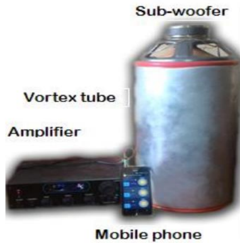
Fig: 3.2 : Portable fire extinguisher
