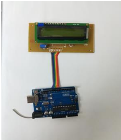
Fig 4.2. Character green backlight - LCD display
