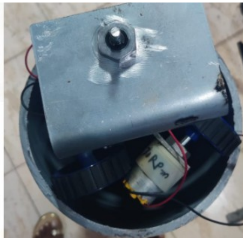
Fig 4.4: 30 RPM DC Motors attached to the wheel
