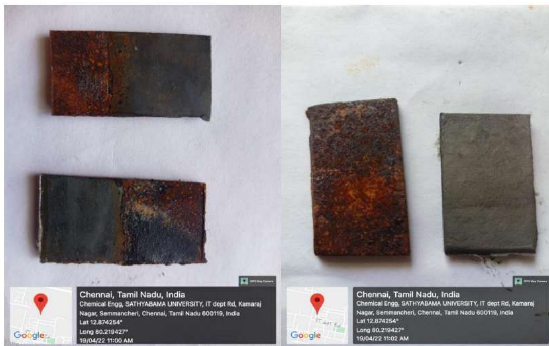
Fig: 5.8 coated metal plate immersed into acid
