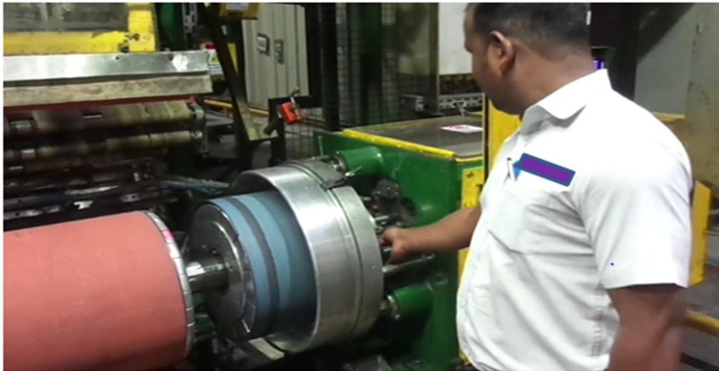
Figure 5.5 : Checking Air Leakage Manually
