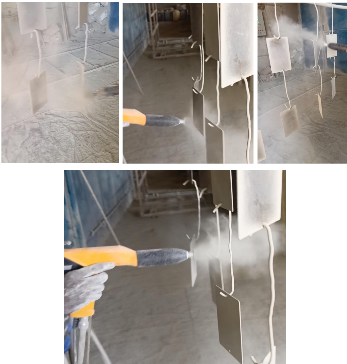
Fig: 4.14: Powder coating of nanoparticles mixed with epoxy on mild steel surface with high pressure spray gun
