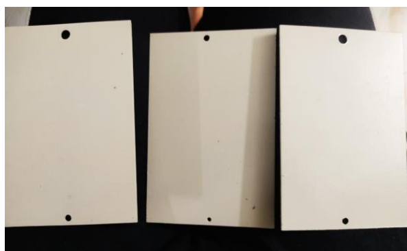
Fig9 and 10 fig9 represents nanoparticle based antifouling coating which is Epoxy Fig10 represents without nanoparticle its only antifouling coating for control.
