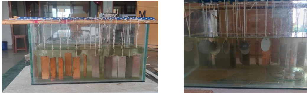
Fig:1 Above pictures are copper slide, stainless steel slide, glass slide, small and big coupons. They are immersed in tank containing seawater. The apparatus leaves for 2-3 days for formation of biofilm.
