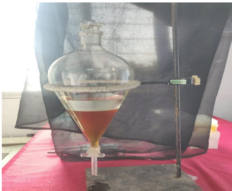
Fig. 4.6: The above picture shows the separating funnel –separation of the secondary metabolite from other biomolecules like fats, lipids
