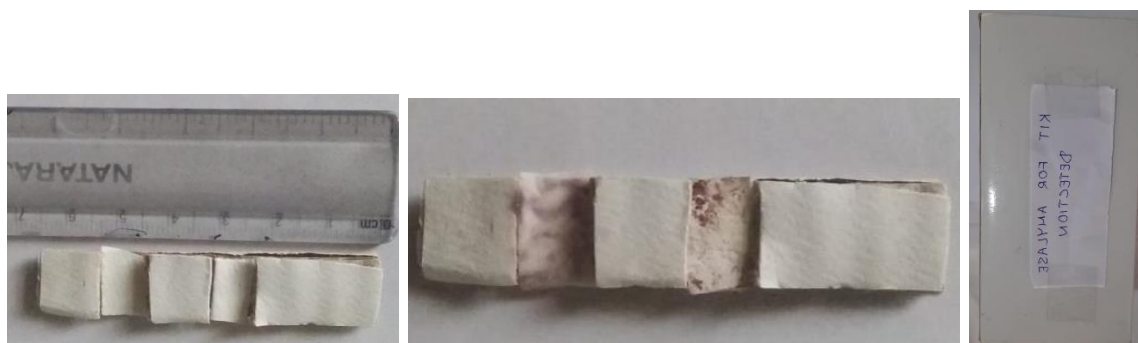
Fig.6. Paper based device for detection of saliva samples
