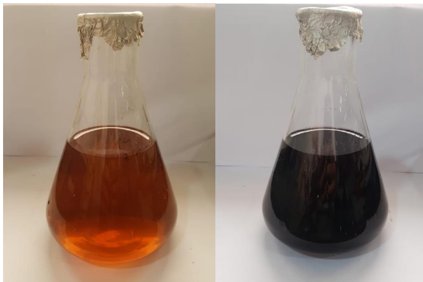
FIGURE 4: 1) after mixing sample and gold chloride solution. 2) formation of gold nanoparticles after 1hr after mixing.
