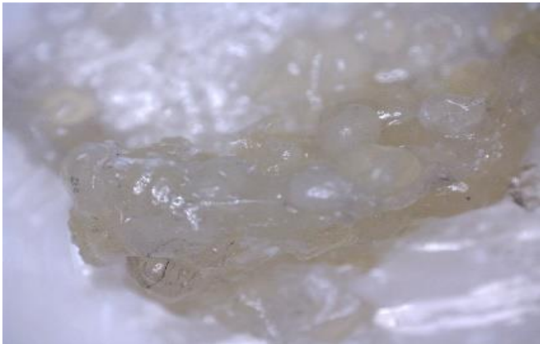
Figure 5.7: Right side view of traditional porous scaffold
