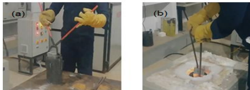
Fig. 4.4: Casting of Mg REE alloys (a) Placing pure magnesium in Stainless Steel Crucible and (b) Placing of stainless-steel crucible in the Electrical resistance furnace
