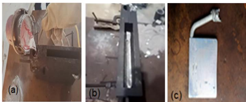
Fig. 4.9: (a) Pouring the alloy molten metal into the preheated die cast steel mold, (b) Shrinkage during the cooling process and (c) As cast Mg Sr Gd alloy
