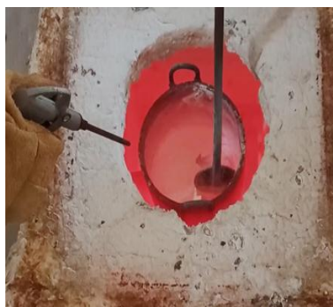
Fig. 4.5: Skimming under protective atmosphere
