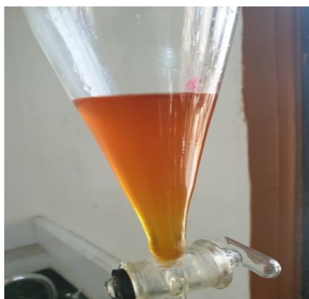
Fig 4.4Transesterification of mixed Biodiesel
