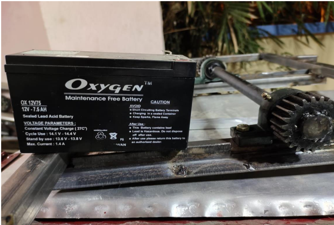
FIG 4.2 LEAD ACID BATTERY
