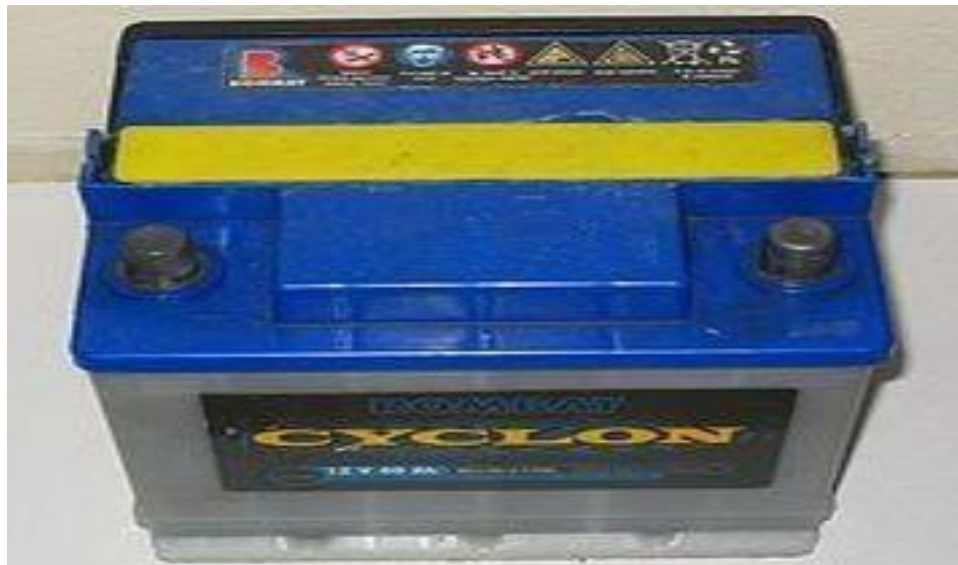
FIG 4.1 LEAD ACID BATTERY PACK
