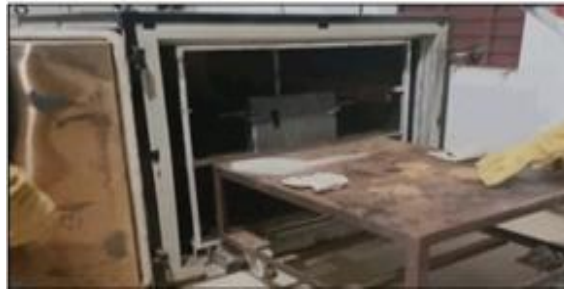
Fig. 4.7: Removal of pre heated die cast steel mould from pre heated Owen
