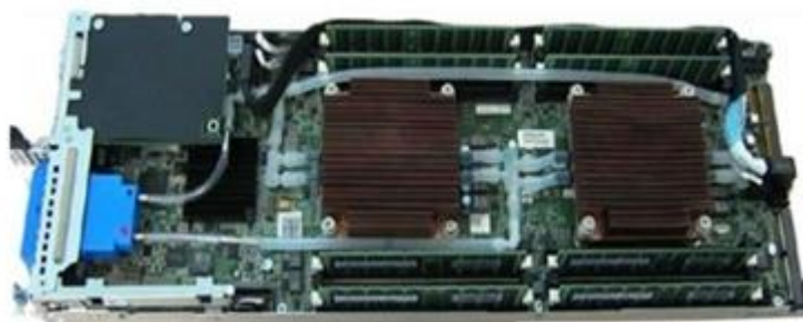
Fig.4.7: Plastic piping in negative pressure liquid
