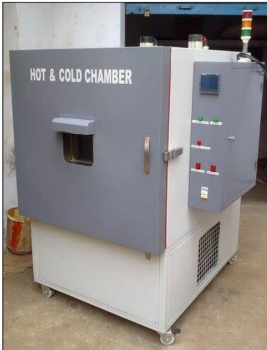
Fig 1.18 Thermal cyclic fatigue test chamber
