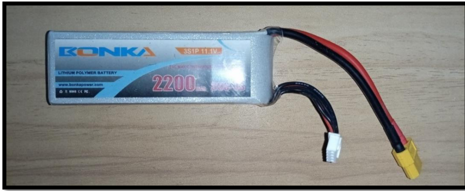
Fig:4.4 : Lithium-Ion Polymer Battery
