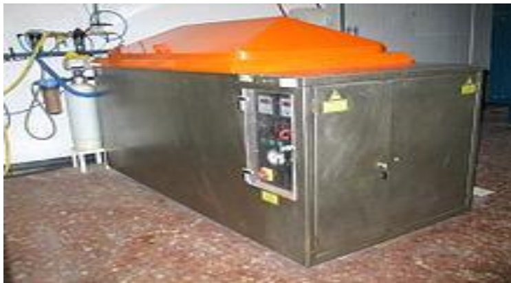
Fig:1.3:A salt spray cabinet
