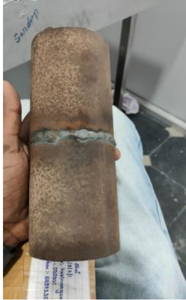
Fig:4.3:TIG Welded pipe
