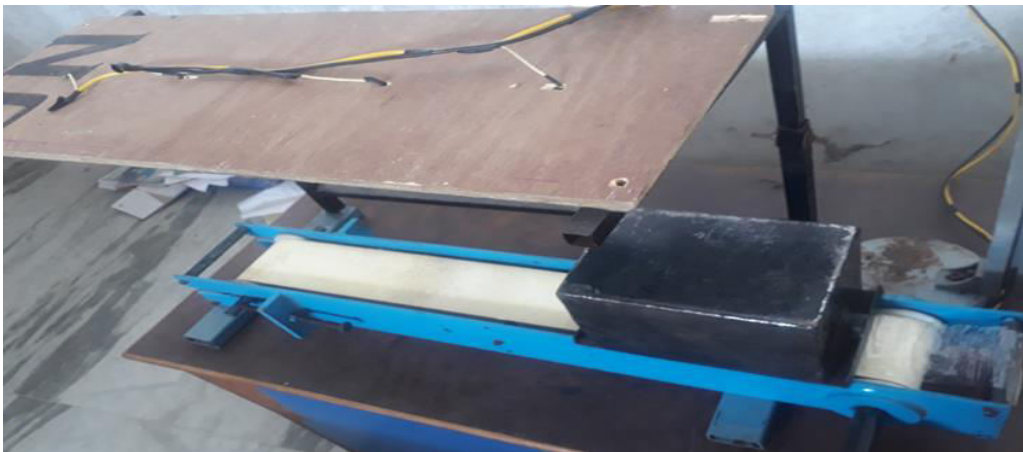
Fig: 4.3: Drying of edible films using infrared radiation plus hot air
