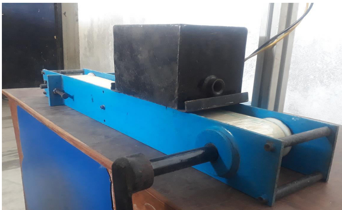
Fig: 4.1: Drying of edible films using hot air blowing
