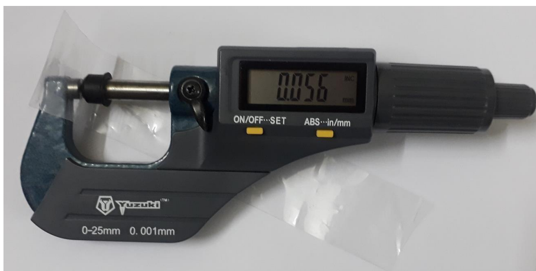
Fig:4.2: Measuring the film thickness of a sample edible film
