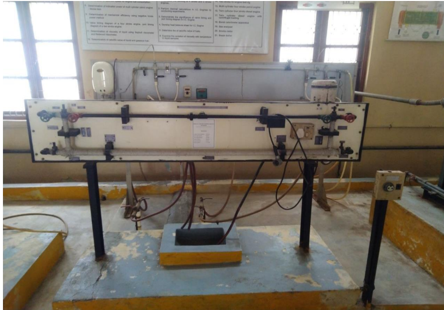
Fig: 3.6: Experimental Setup of Double Pipe Heat Exchanger
