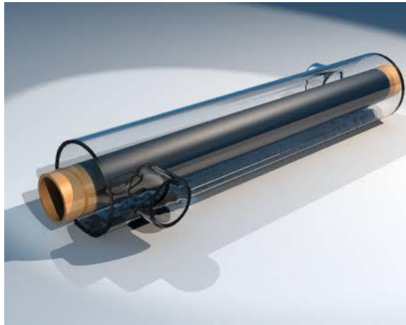
Fig: 3.10: Pilot-Scale Double Pipe Heat Exchanger Geometry
