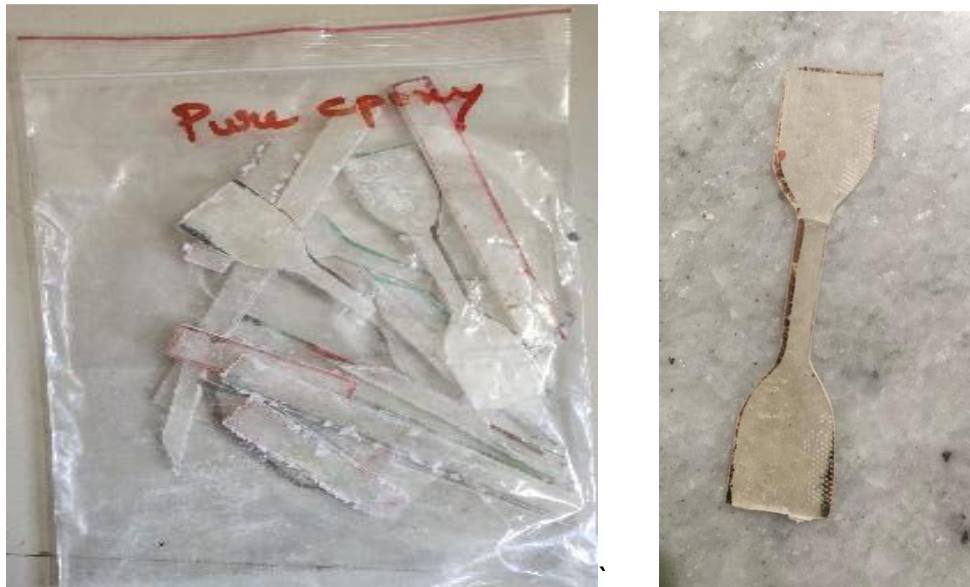
Fig:5.1: Tensile samples of pure Epoxy
