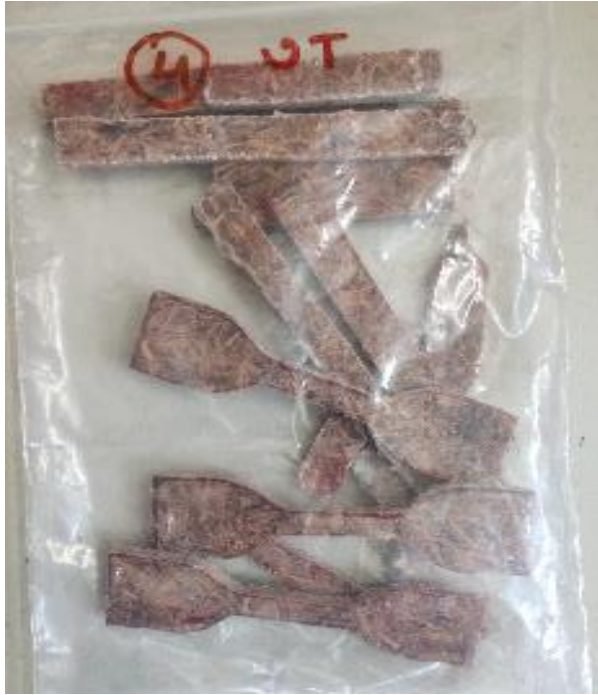
Fig:5.2: Tensile samples of untreated banyan roots fiber composite
