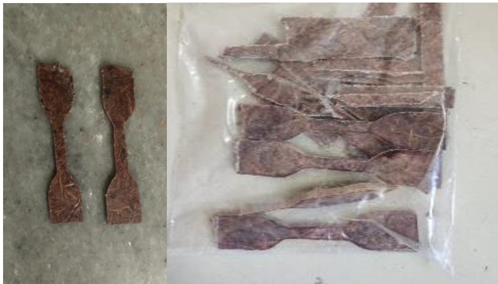
Fig:5.3: Tensile samples of treated banyan roots fiber composite
