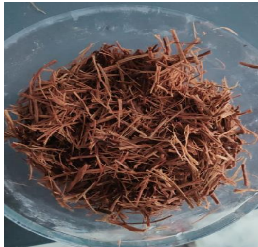
Fig:4.6: Fiber treated with 10 % \text{Ca}(\text{OH})_2 chemical
