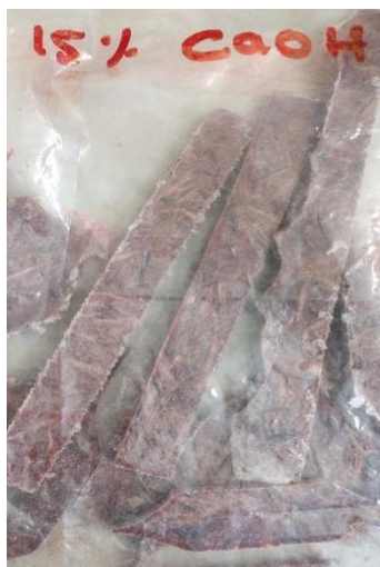
Fig:5.6: Flexural samples of Epoxy + Treated banyan root fiber
