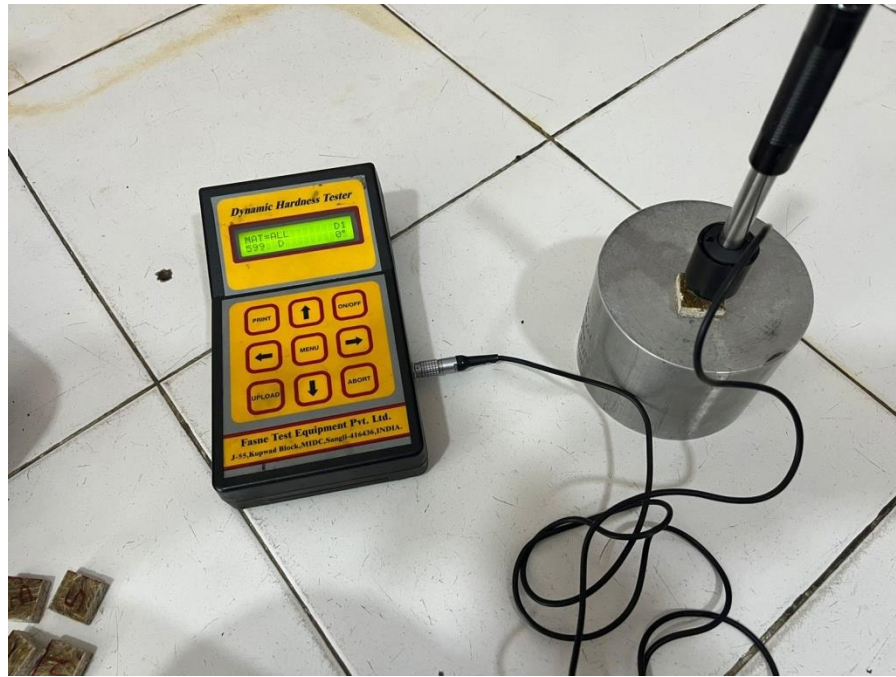
Fig 4.1: Shour D hardness
