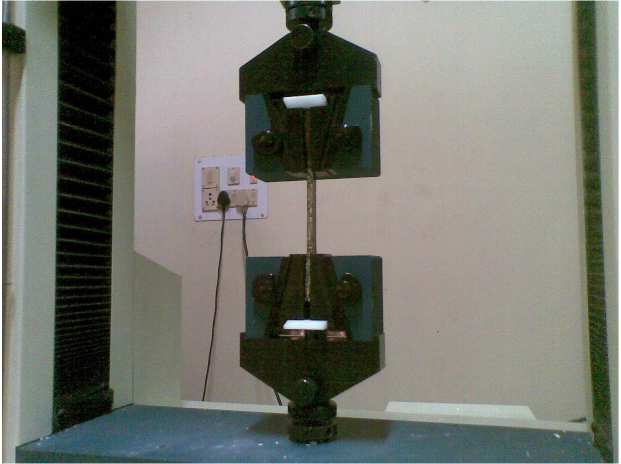
Figure (4.6) UTM machine tensile testing sample loading condition.
