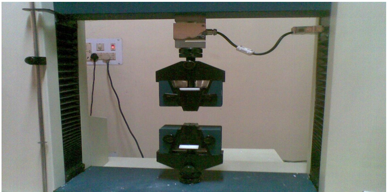
FIG(4.5) Sample unloaded for tensile testing on the UTM machine.
