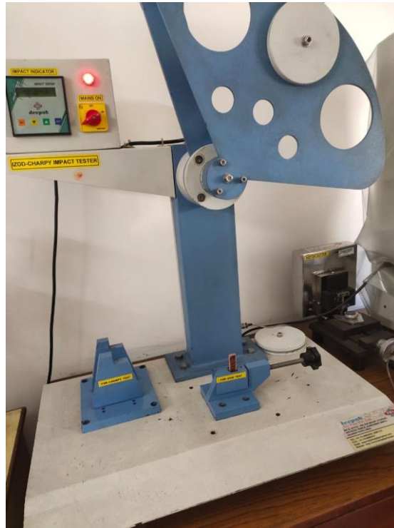
Figure 4.11: Izod Impact Testing Machine
