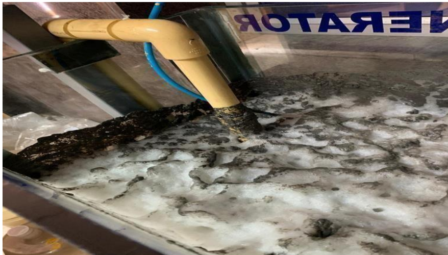
Fig 4.7 Micro Nano Bubble Generator Contains Laundry Water With Thethankotai Powder
