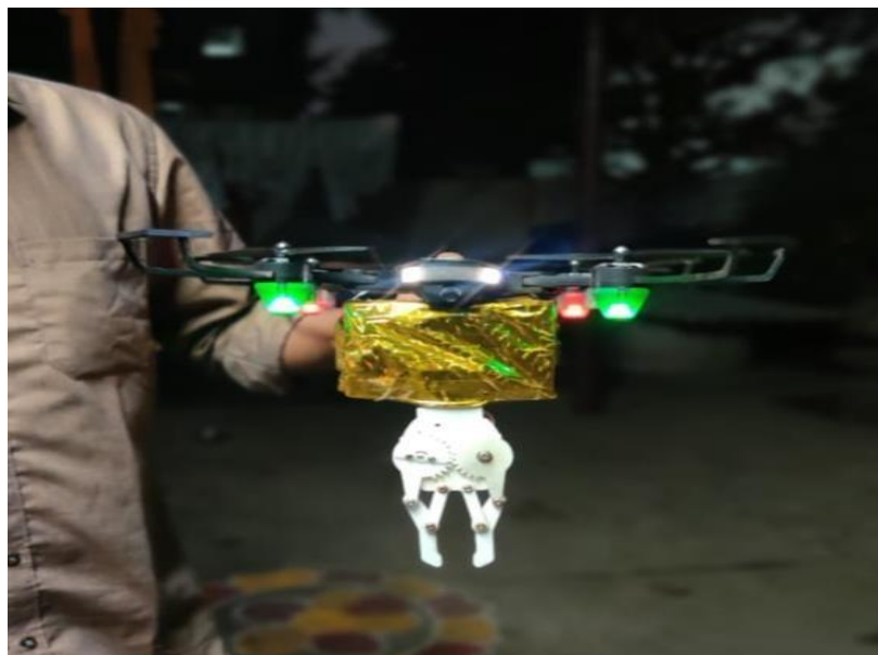
Fig 5.1: Assembled Drone with Gripper mechanism
