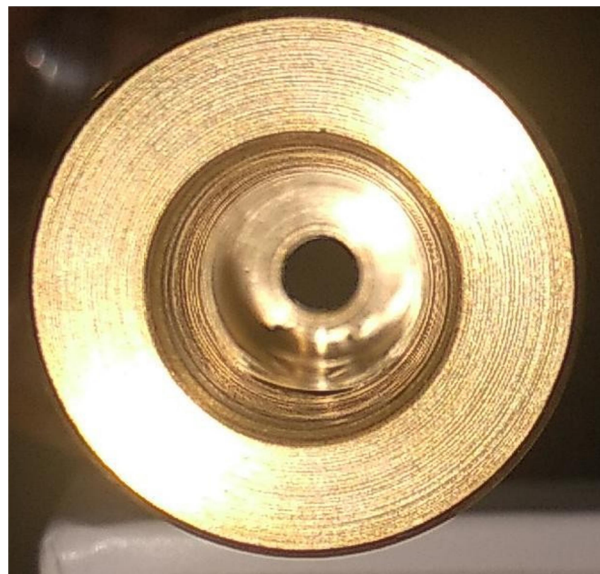
Figure 5.2: Fabricated venturi design (Cross-sectional view)
