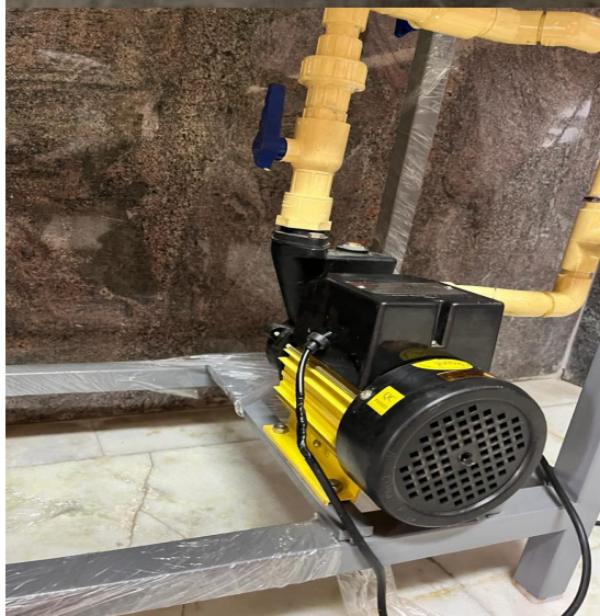
Fig : 4.2: Equipment for nanobubble generation
