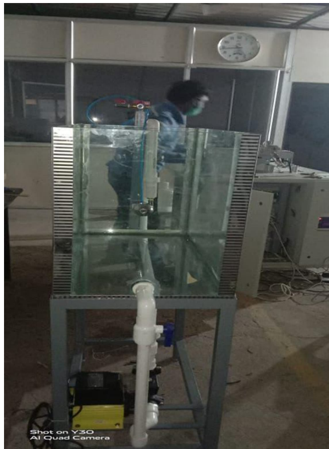
Fig: 4.2: Equipment for generating Nanobubbles
