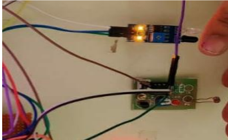
Fig:5.10 : LDR detects low light and IR detects movement
