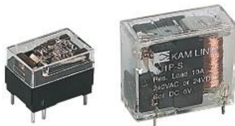
fig no.5.2ELECTRICALOPERATED SWITCH
