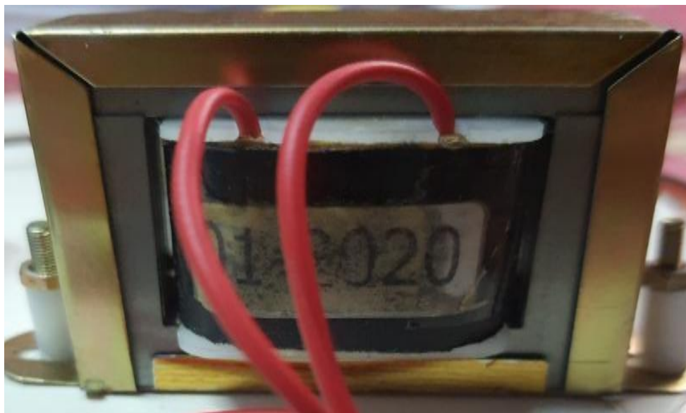
Figure 3.15 –The Step down Transformer
